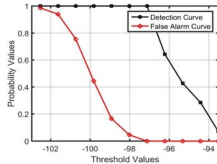
Figure 6: Performance for the Signal plus Noise dataset for (SNR=10dB to 1dB)
