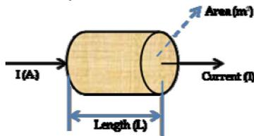
Figure 1: Current flow through a uniform cylindrical soil (adapted from [5]).
